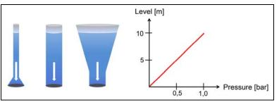
Figure 1: Illustration of the hydrostatic paradox
