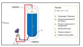
Figure 9: Hydrostatic level measurement using differential pressure sensors
