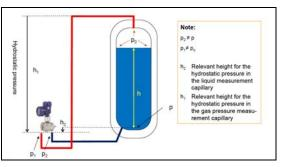
Figure 10: Effects of positioning on differential pressure sensors in level measurement
