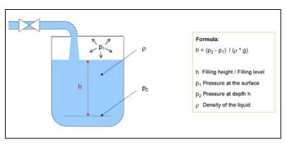
Figure 3: Level measurement in sealed, gas-tight tanks and vessels
