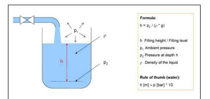
Figure 2: Level measurement in open, vented tanks and vessels
